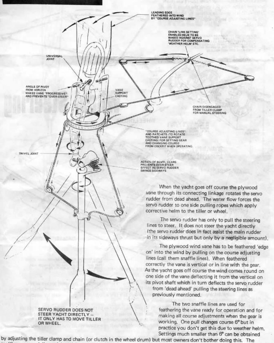
snaffles are especially useful at night as you can make any course adjustments by simply pulling once or twice etc. and have some idea of what you will get (unlike a wormwheel and endless cord),
